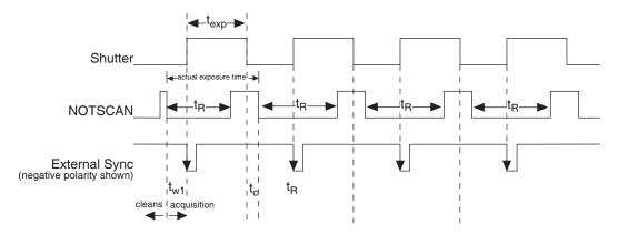
Figure 17. Frame Transfer where  $t_{w1+}$   $t_{exp} + t_c > t_R$
